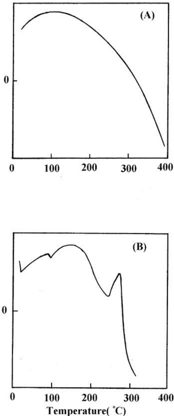
**Figure 2.** DSC profile, (A) lignin , (B) copolymer vertical coordinate: Heat flow,  $\uparrow$ ,  $>0$  abscissa: Temperature( $^{\circ}\text{C}$ )
