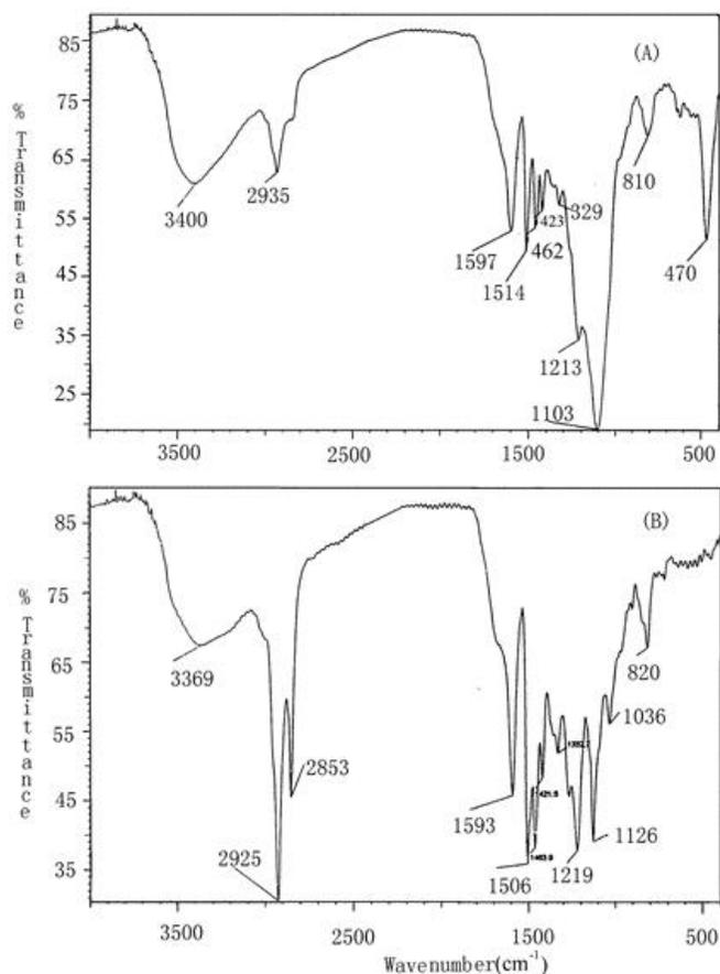
**Figure 1. FTIR spectra , (A) FTIR spectrum of copolymer, (B) FTIR spectrum of lignin vertical coordinate: Relative transmittance abscissa: Wavenumber( $\text{cm}^{-1}$ )**
