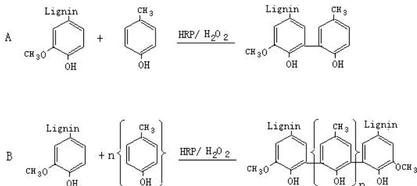
**Figure 3. Reaction for HRP catalyzed copolymerization of lignin with cresol**
