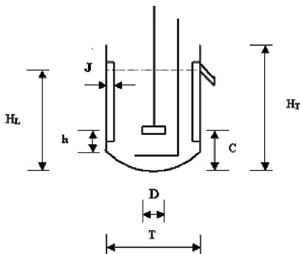
Figure 1. Schematic representation and main dimensions of the 5 L continuous stirred tank reactor.
