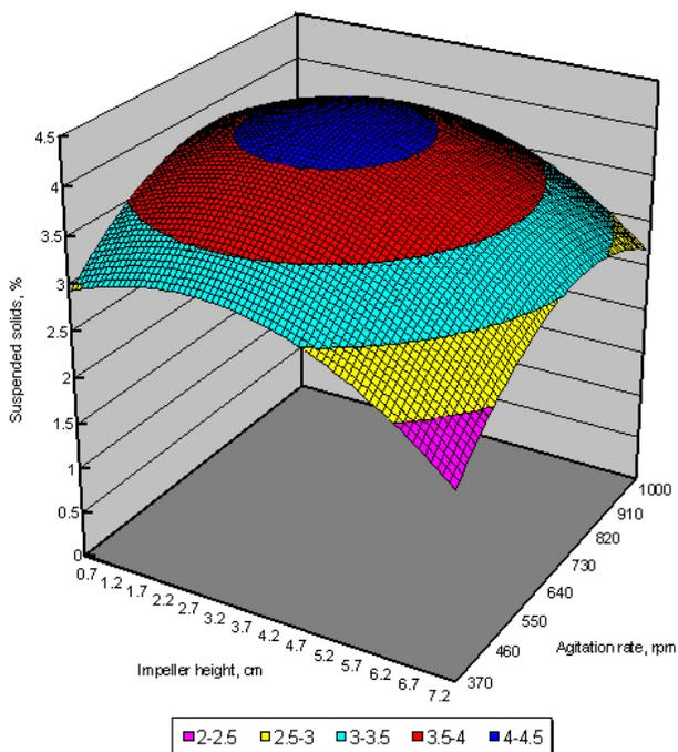
**Figure 2. Solids concentration in the exit stream as a function of impeller position and agitation rate in the case of the 3MPU impeller, 6% w/v pulp density, 2.0 vvm.**
