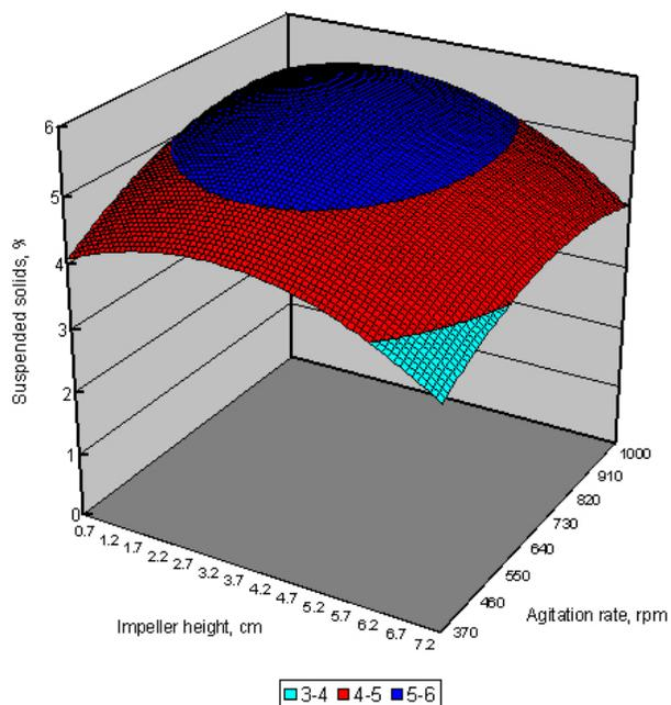
**Figure 3. Mean solids concentration in the tank as a function of impeller position and agitation rate in the case of the 3MPU impeller, 6% w/v pulp density, 2.0 vvm.**
