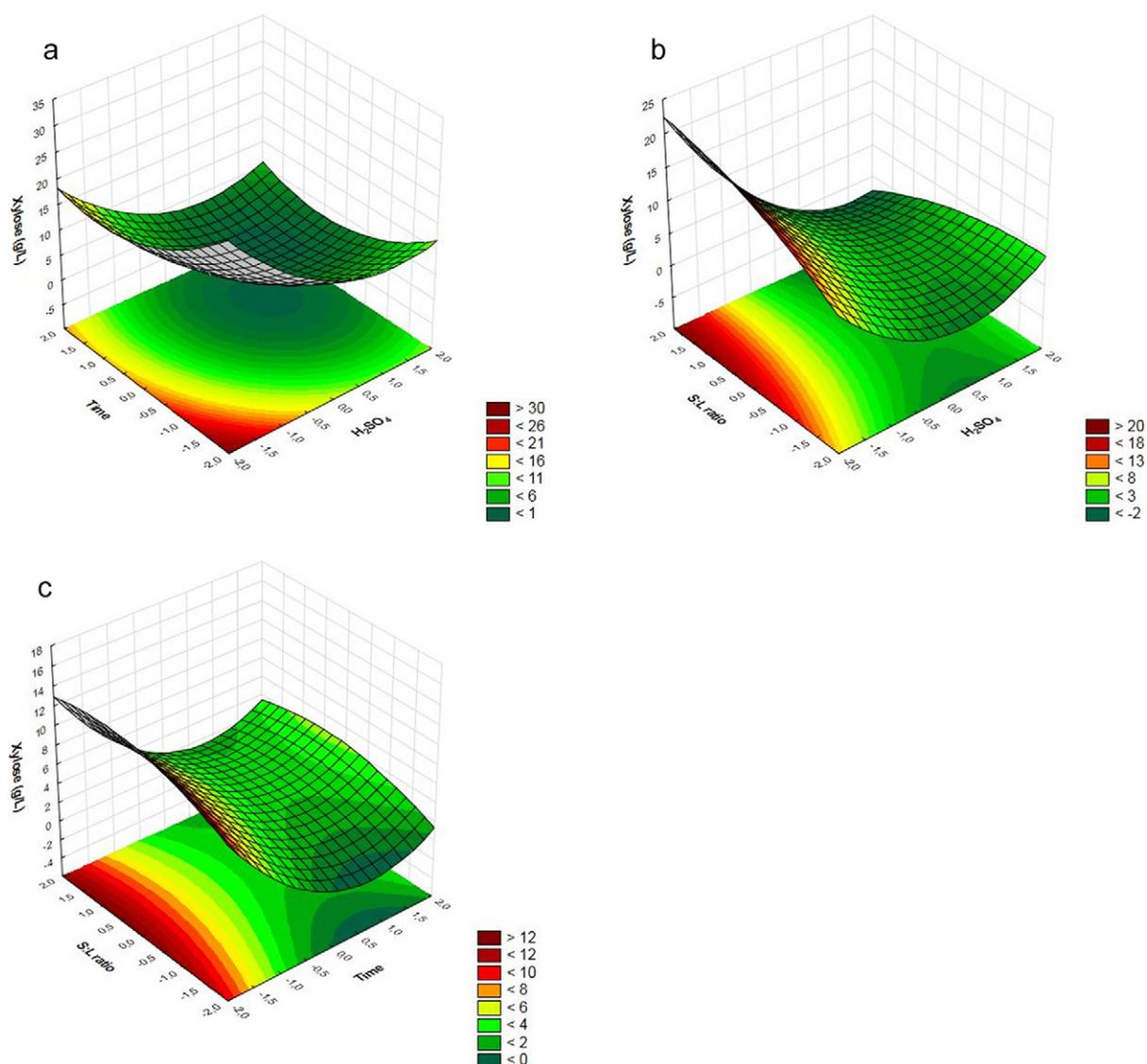
**Fig. 3.** Response surface for the xylose concentration in the hydrolysates from the solid fraction obtained from the alkaline pretreatment after the acid pretreatment as functions of the following variables: (a) sulfuric acid concentration and exposure time and (b) sulfuric acid concentration and solid-to-liquid ratio (c) exposure time and solid-to-liquid ratio.
