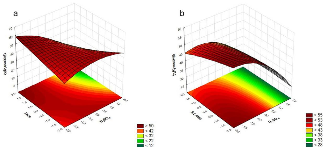
**Fig. 2.** Response surface for the glucose concentration in the hydrolysates from the solid fraction obtained from the alkaline pretreatment after the acid pretreatment as functions of the following variables: (a) sulfuric acid concentration and exposure time and (b) sulfuric acid concentration and solid-to-liquid ratio.
