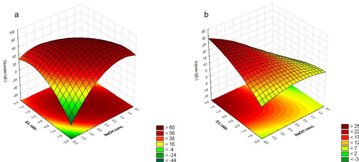
**Fig. 4.** Response surface for the glucose (a) and xylose (b) concentration in the hydrolysates from the solid fraction obtained from the alkaline pretreatment as functions of variables sodium hydroxide concentration and solid-to-liquid ratio.
